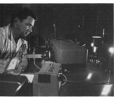
MONOCHROMATOR ANALYZER is used by Ed Machin to evaluate light detector device. The monochromator's prisms isolate thin wave lengths of light which are used to compare against the device performance.
